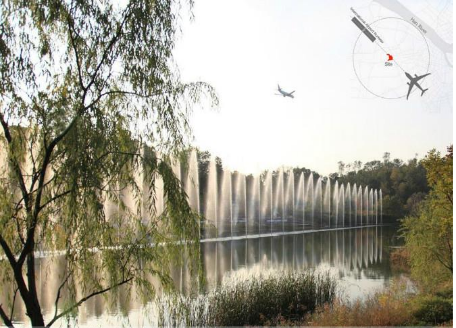
The lake contains 41 vertical fountain jet nozzles that automatically activate when the aircraft noise level exceeds 61 decibels. The sound of the water shooting from the fountain helps offset the aircraft noise overhead, a common occurrence because of the park's location near International Airport. This fountain takes usage of the noise pollution that causes inconvenience on the part of citizens and transforms it into the motivation of an event, emphasizing the main theme of the park, "rebirth".
